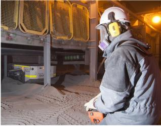
Designed and built by MINPROVISE, the DUGLESS 900 is an automated digging and cleaning unit capable of safely maneuvering under low conveyor sections and other inaccessible places to remove spillage and blockages without any risk to workers or equipment.
