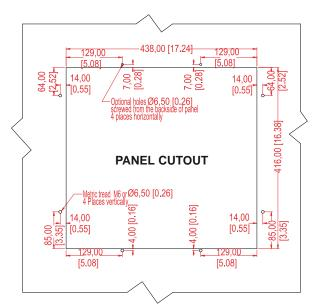
Dimensions might be shown with or without decimals and indicated as mm [inches]. Tolerance on drawings is +/- 1mm. For accurate measurements, check relevant DWG file.
